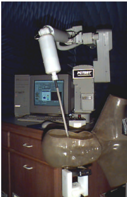
Figure 5. Photograph of the Probe and the Phantom
