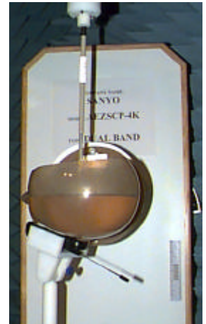
Fig. 1 SAR Test Set-up
