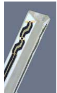
Figure 3.2 Probe Thick-Film Technique
