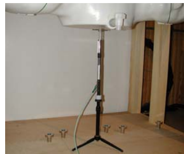
Figure 12.1 Dipole Validation Test Setup
