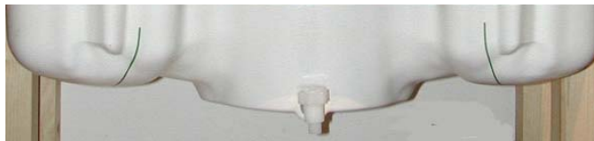
Figure 7.2 SAM Twin Phantom shell
