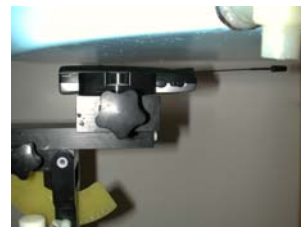
Figure 19. Body/Mouth SAR Test Setup
