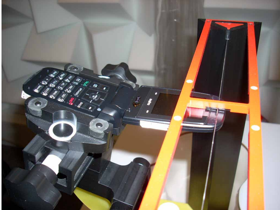
Figure 17-1 Ear Reference Point HAC Phantom Alignment
