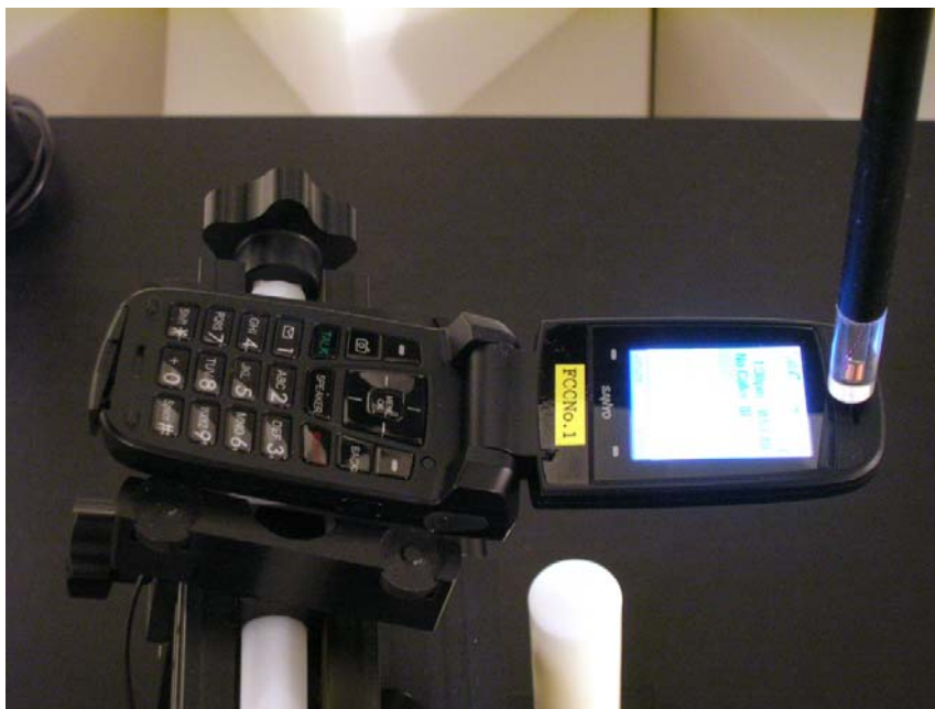
Figure 0-1 Test Setup for Wireless Device
