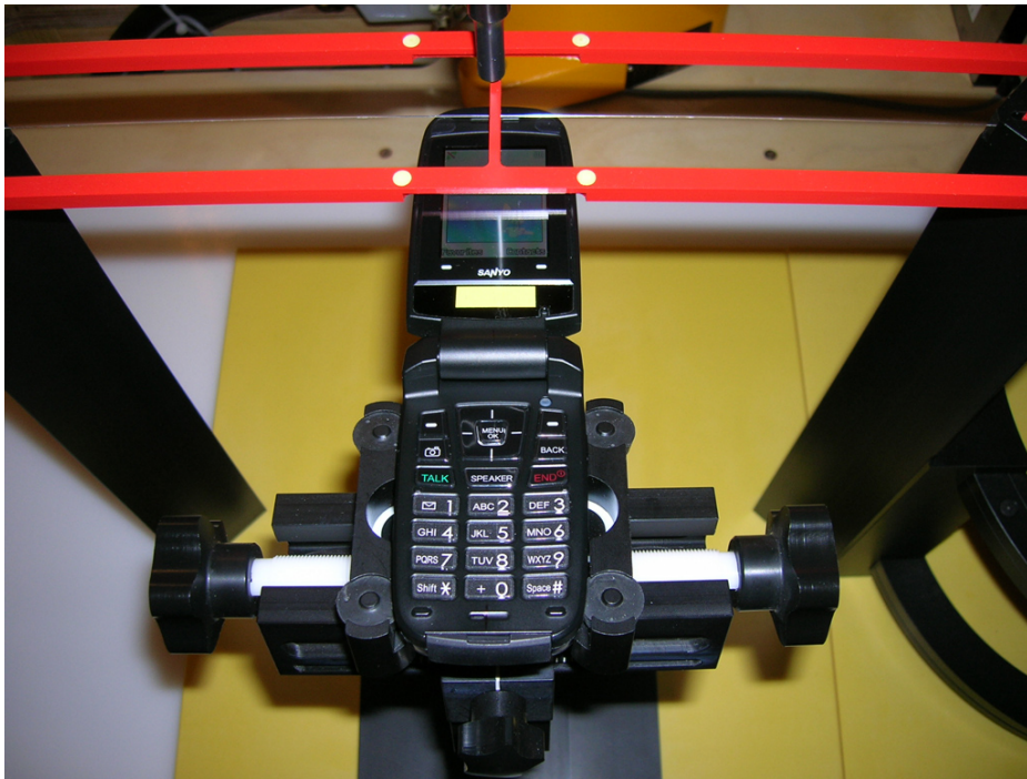
Figure 17-2 HAC Phantom Plane Alignment
