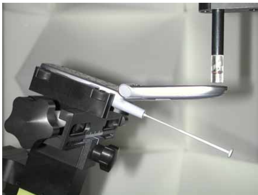
Figure 0-2 Test Setup for Wireless Device
