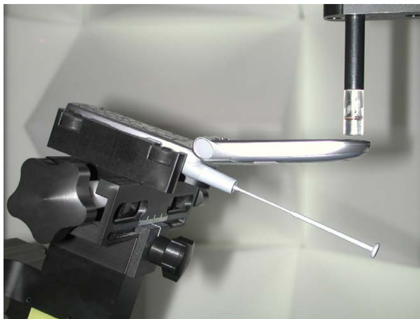
Figure 13-2 Test Setup for Wireless Device
