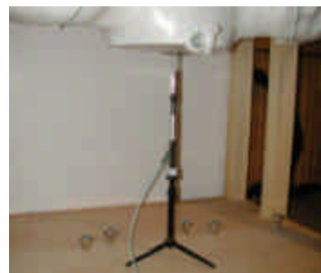
Figure 12.1 Dipole Validation Test Setup
