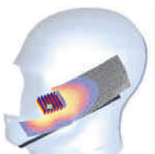
Figure 7.1 Sample SAR Area Scan
