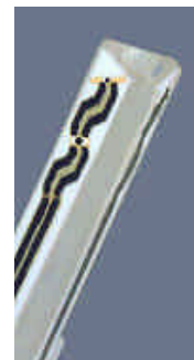
Figure 3.2 Probe Thick-Film Technique
