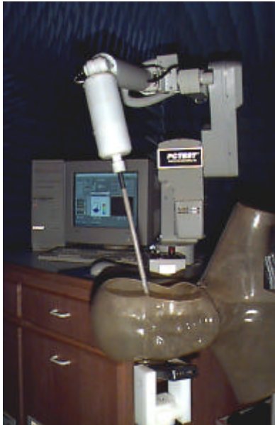
Figure 5. Photograph of the Probe and the Phantom
