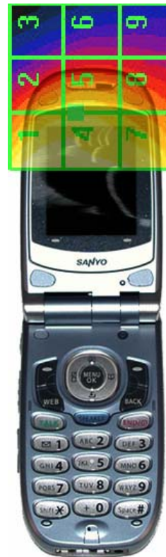
Figure 31 H-Field WD Scan overlay
