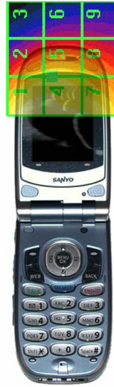
Figure 33 H-Field WD Scan overlay
