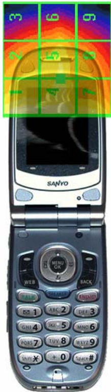
Figure 32 E-Field WD Scan overlay
