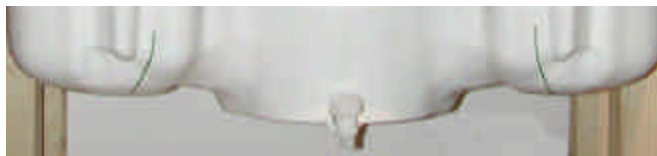
Figure 7.2 SAM Twin Phantom shell
