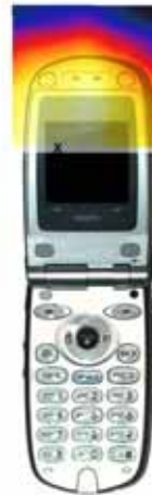
Figure 27 Sample E-field Scan Overlay
