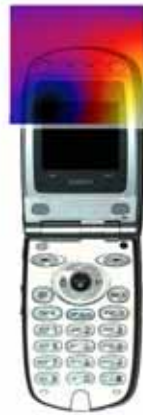
Figure 28 Sample H-field Scan Overlay
