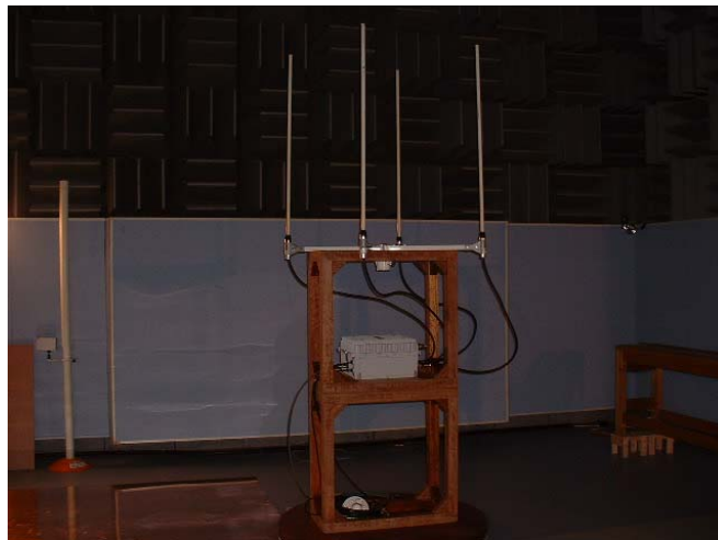
Side View(Transmitter Antenna System: ANT5-ANT8)
