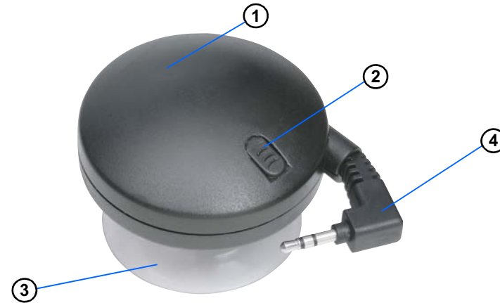
Figure 9: TMC antenna with take up reel
