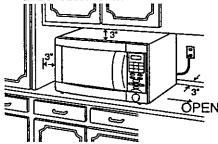
A minimum clearance of 3 inches is required between the oven and any adjacent wall. One side must be open.
