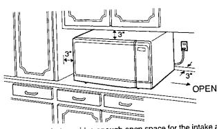
1. Select a level surface that provides enough open space for the intake and/or outlet vents.
