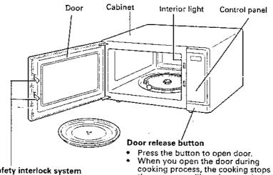
Safety interlock system Shuts off oven power if door is opened during operation.
