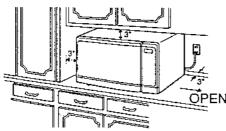
A minimum clearance of 3 inches is required between the oven and any adjacent wall. One side must be open.
