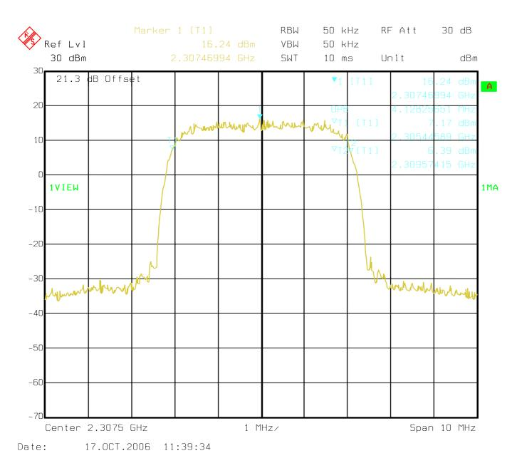
Plot 2 - Occupied bandwidth (99%, channel A, 2307.5 MHz)
