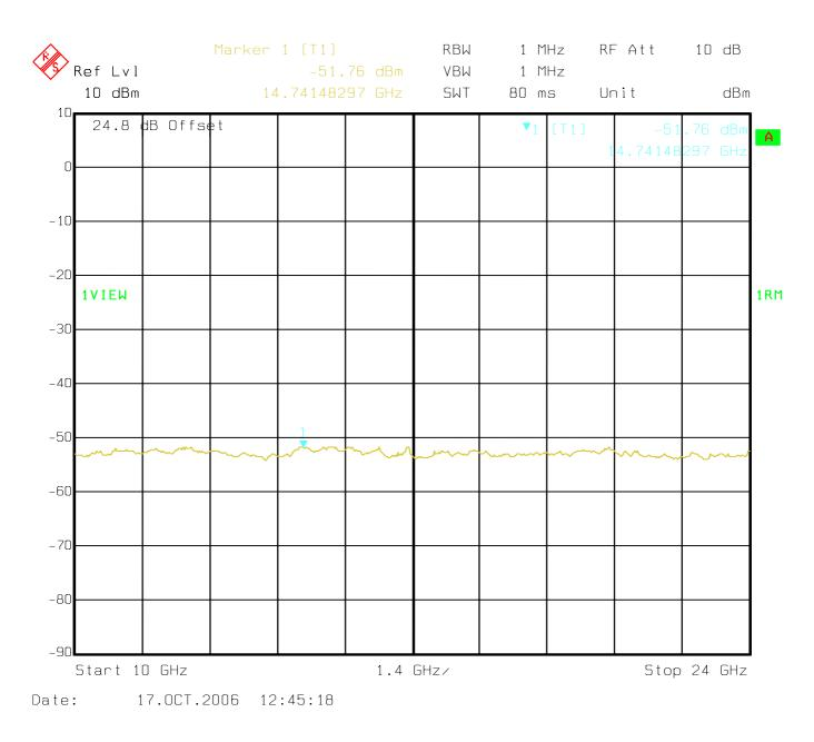
Plot 12 - Spurious emissions at the antenna terminals (10 GHz to 24 GHz, channel B, 2312.5 MHz)
