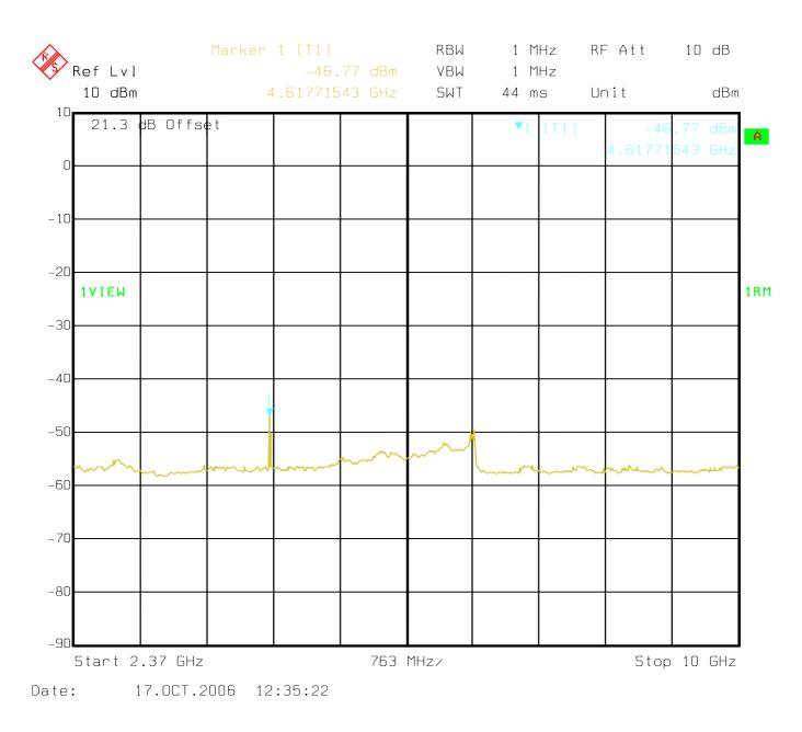
Plot 11 - Spurious emissions at the antenna terminals (2370 MHz to 10 GHz, channel B, 2312.5 MHz)
