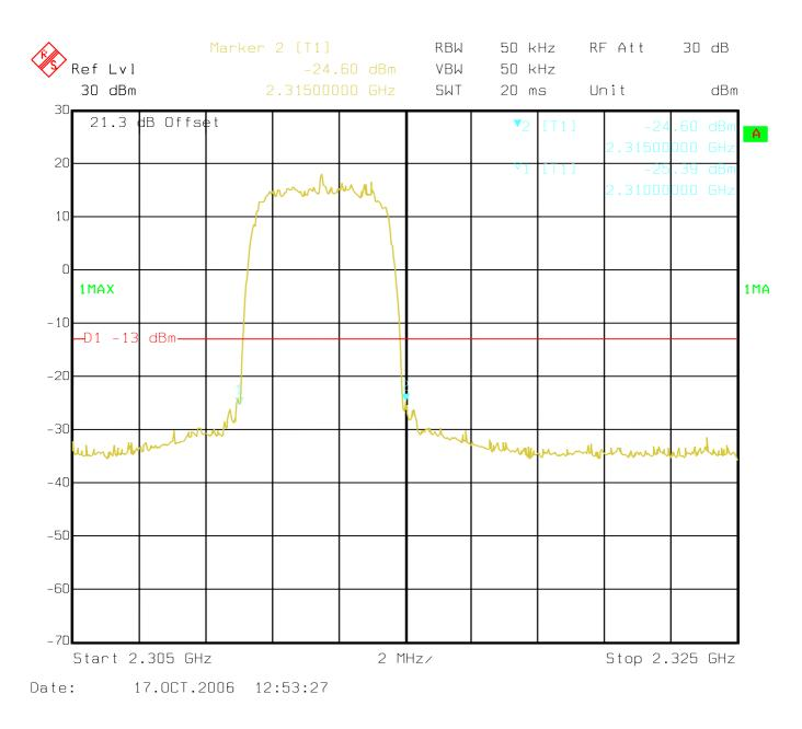
Plot 14 - Spurious emissions (bandedges) at the antenna terminals (2305 MHz to 2325 MHz, channel B, 2312.5 MHz)
