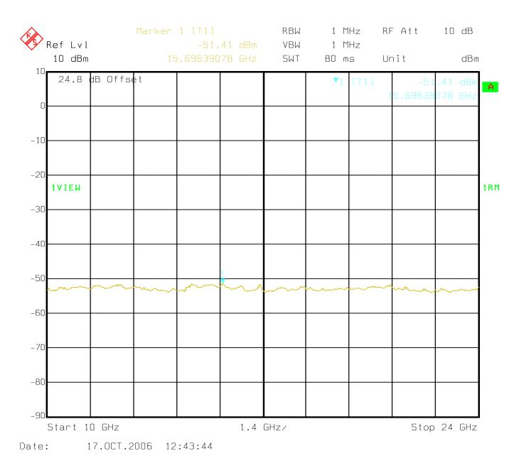
Plot 9 - Spurious emissions at the antenna terminals (10 GHz to 24 GHz, channel A, 2307.5 MHz)
