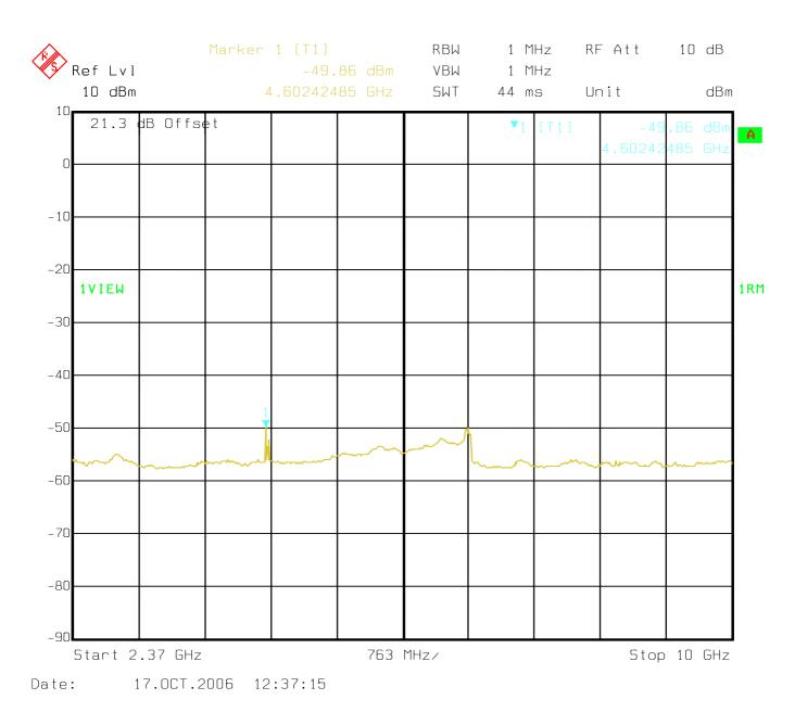
Plot 8 - Spurious emissions at the antenna terminals (2370 MHz to 10 GHz, channel A, 2307.5 MHz)
