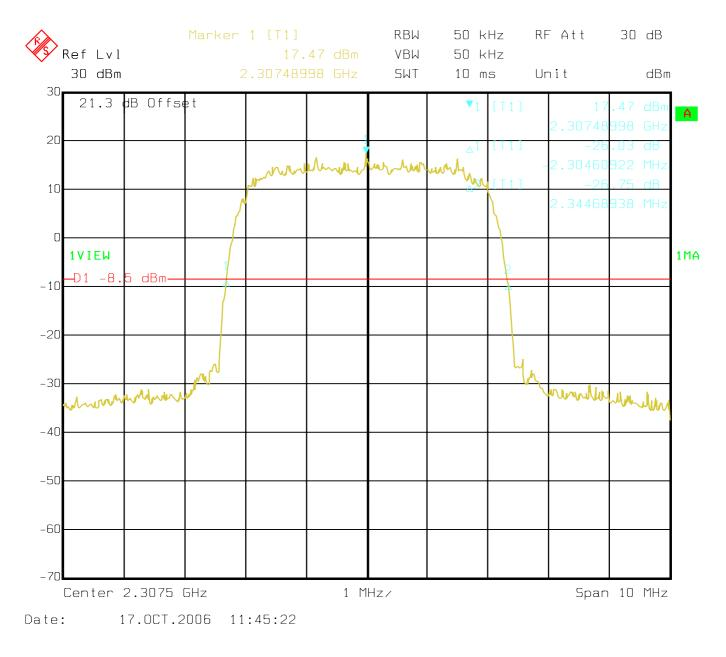
Plot 1 - Occupied bandwidth (-26 dB, channel A, 2307.5 MHz)
