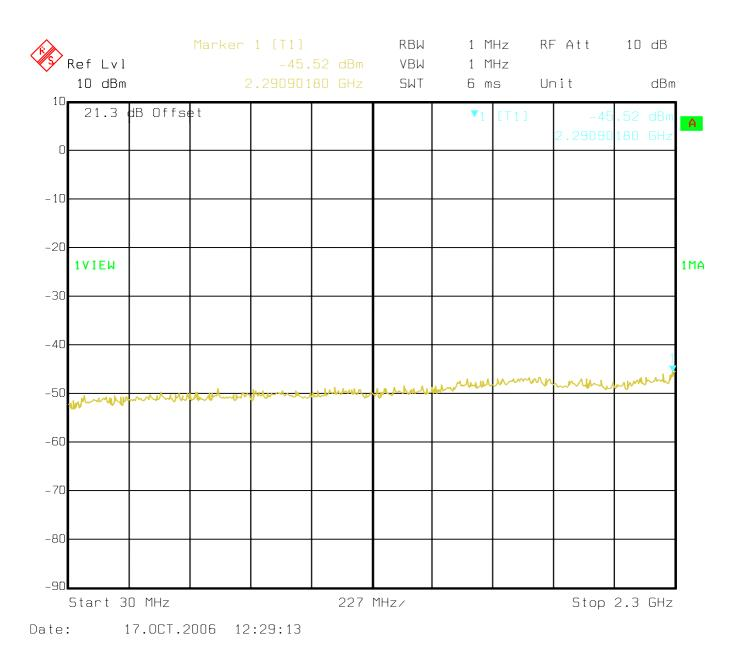
Plot 10 - Spurious emissions at the antenna terminals (30 MHz to 2300 MHz, channel B, 2312.5 MHz)
