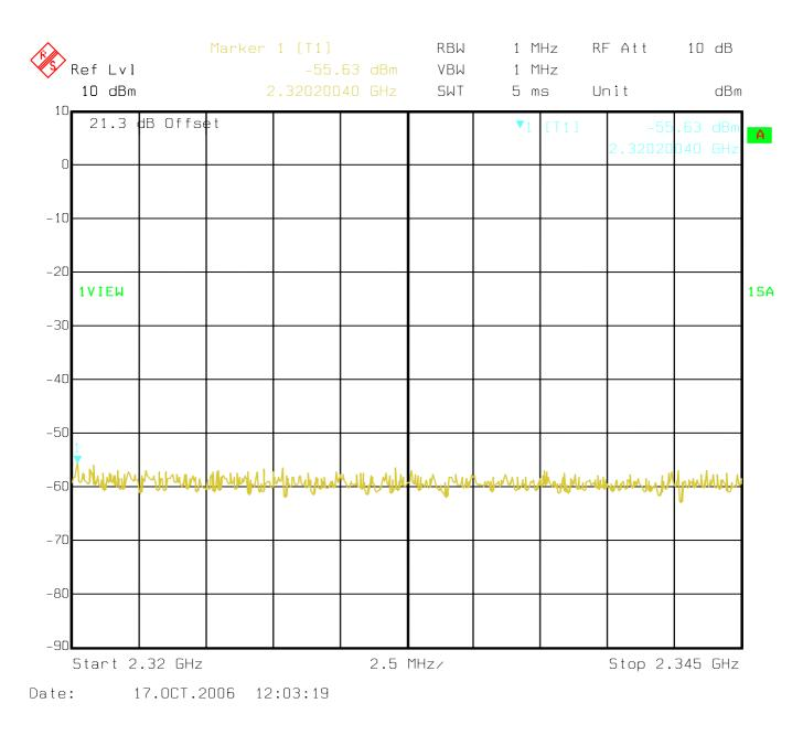
Plot 6 - Spurious emissions at the antenna terminals (2320 MHz to 2345 MHz, channel A, 2307.5 MHz)
