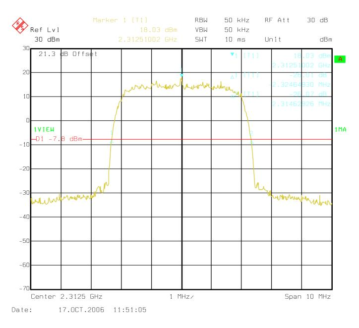
Plot 3 - Occupied bandwidth (-26 dB, channel B, 2312.5 MHz)
