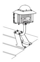
When installing the outdoor unit on a roof, install it in the highest possible location to maximize the signal you receive.
