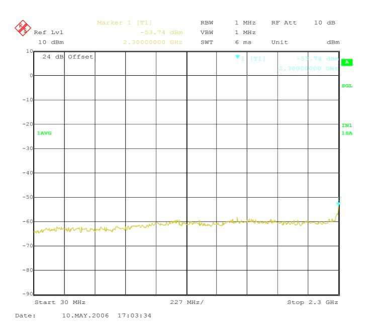
Plot 7 - Spurious emissions at the antenna terminals (30 MHz to 2300 MHz, channel A, 2307.5 MHz)
