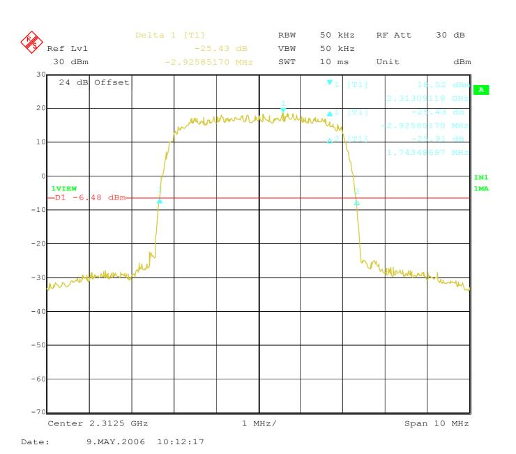
Plot 3 - Occupied bandwidth (-26 dB, channel B, 2312.5 MHz)
