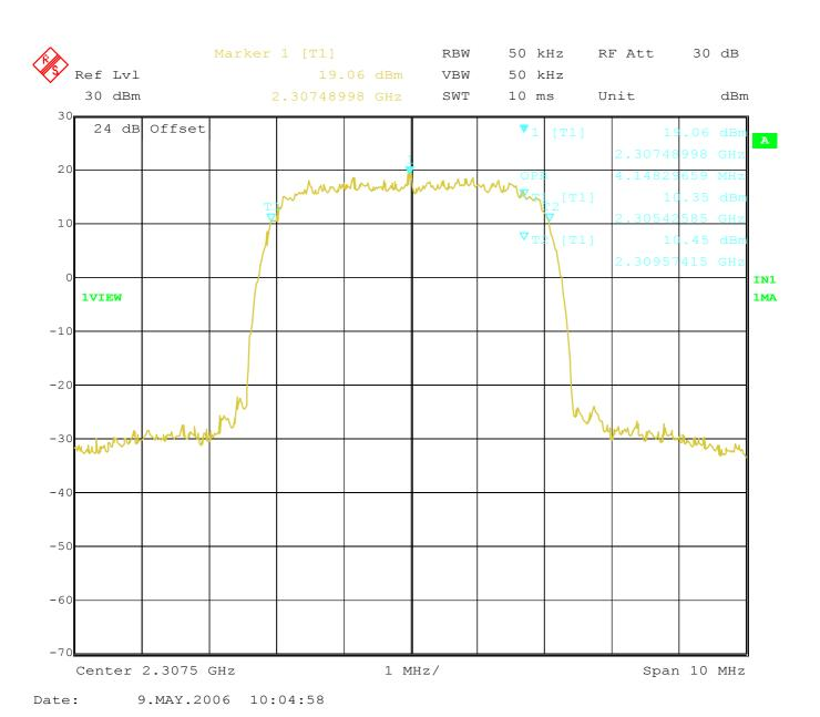
Plot 2 - Occupied bandwidth (99%, channel A, 2307.5 MHz)
