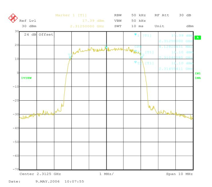
Plot 4 - Occupied bandwidth (99%, channel B, 2312.5 MHz)
