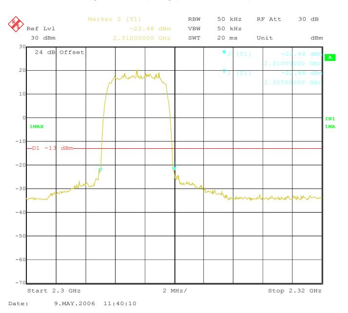
Plot 13 - Spurious emissions (bandedges) at the antenna terminals (2300 MHz to 2320 MHz, channel A, 2307.5 MHz)
