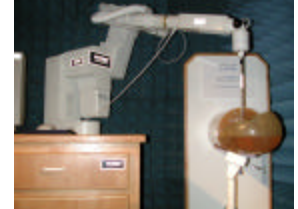
Fig. 1 SAR Test Setup
