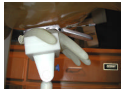
Figure 16. Body SAR Test Setup
