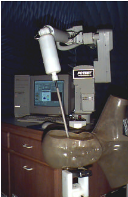
Figure 5. Photograph of the Probe and the Phantom
