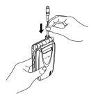
Move it straight down by pulling on a lower part of the antenna.
