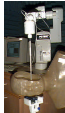
Figure 1. SAR Test Set-up
