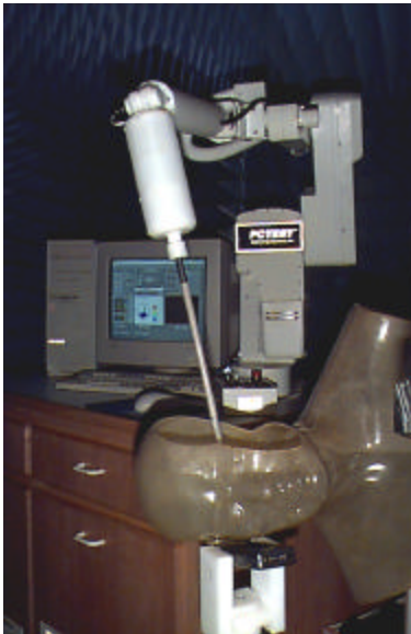
Figure 5. Photograph of the Probe and the Phantom
