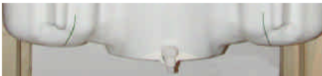
Figure 7.2 SAM Twin Phantom shell
