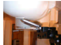
Figure 14.4 Right Head SAR Test Setup -- Ear / Tilt Position --
