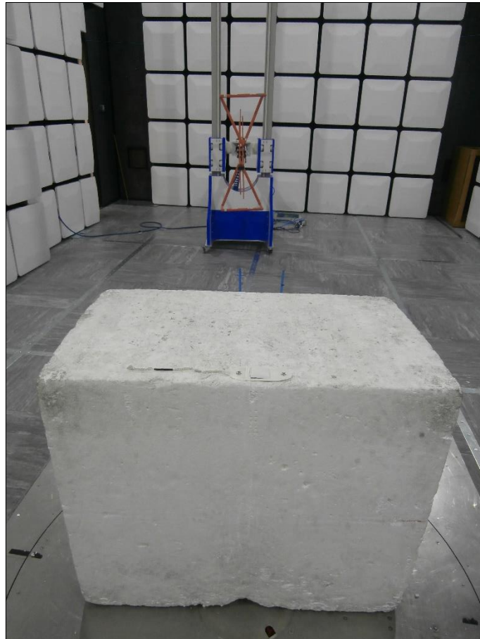
Figure 67 - Test Setup - 30 MHz to 1 GHz - X Orientation
