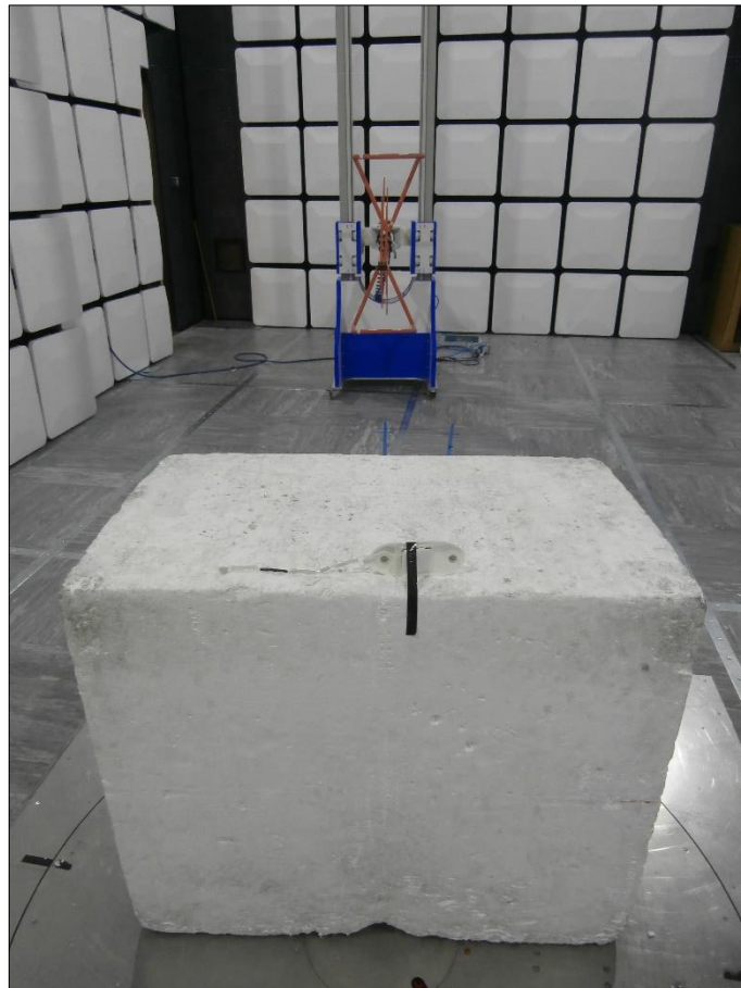
Figure 69 - Test Setup - 30 MHz to 1 GHz - Z Orientation
