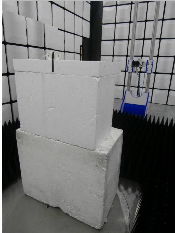
Figure 72 - Test Setup - 1 GHz to 10 GHz - Z Orientation
