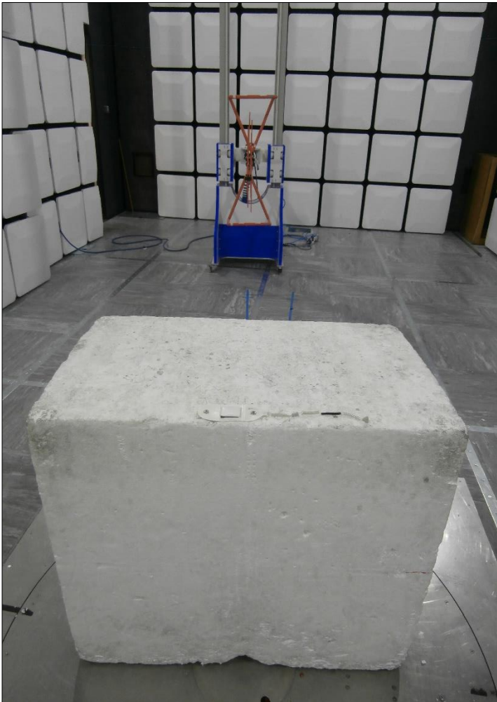
Figure 20 - Test Setup - 30 MHz to 1 GHz - X Orientation
