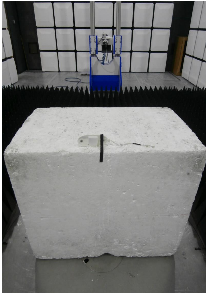
Figure 25 - Test Setup - 1 GHz to 5 GHz - Z Orientation
