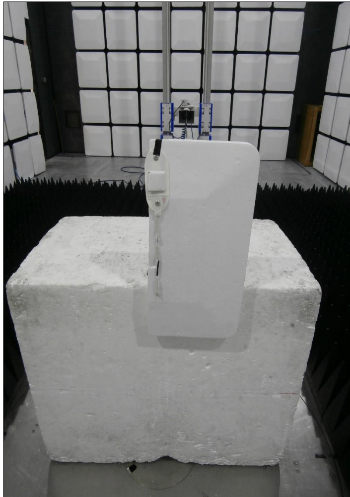
Figure 24 - Test Setup - 1 GHz to 5 GHz - Y Orientation
