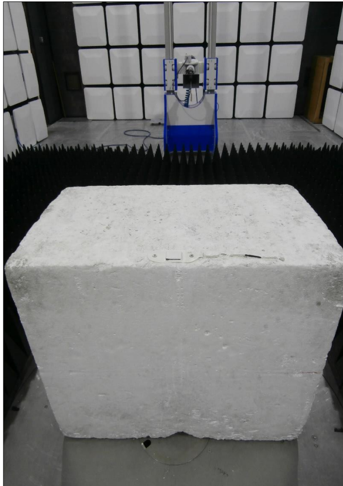
Figure 23 - Test Setup - 1 GHz to 5 GHz - X Orientation
