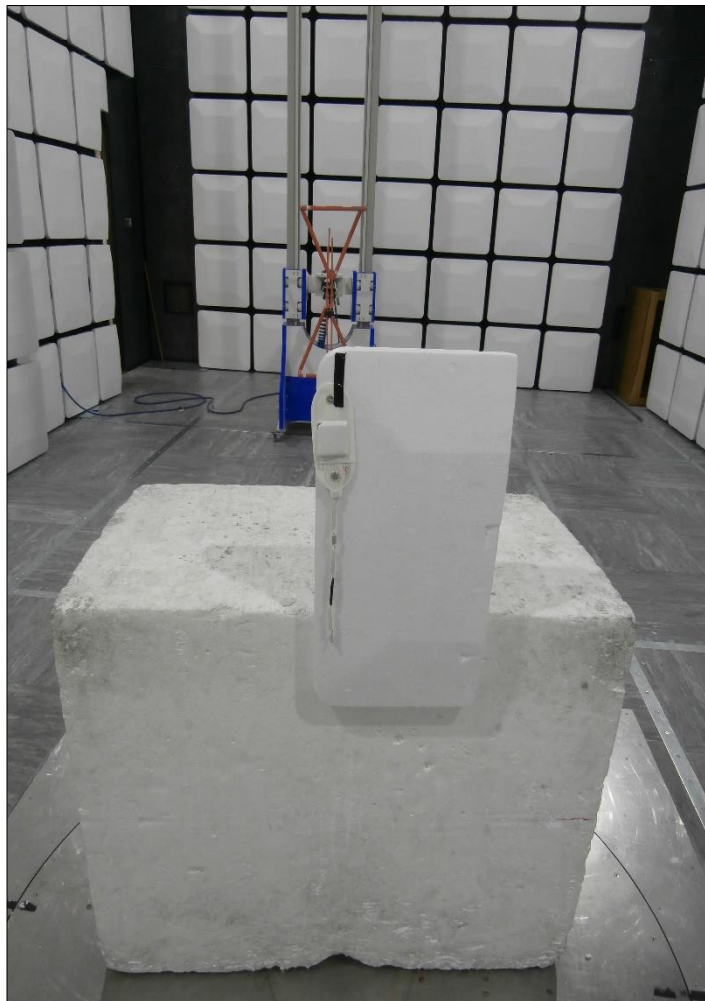
Figure 21 - Test Setup - 30 MHz to 1 GHz - Y Orientation
