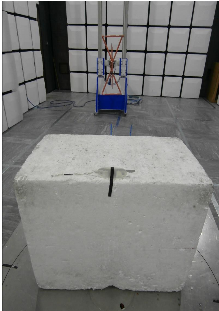
Figure 22 - Test Setup - 30 MHz to 1 GHz - Z Orientation
