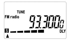
The scanner stops tune if the scanner find the broadcasting station.
