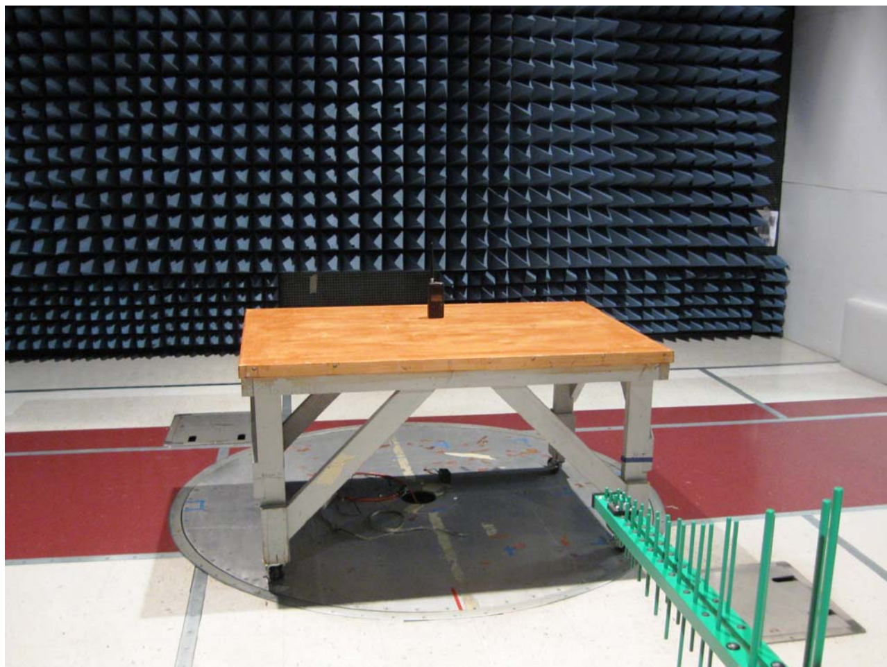
Photograph 4. Radiated Emission Limits Test Setup (30M-1GHz Battery Power test setup)
