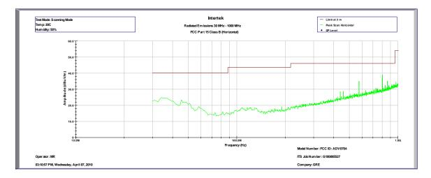
Intertek Testing Services Radiated Emissions 30 MHz - 1000 MHz FCC Part 15 Class B (Pk-Horizontal)
