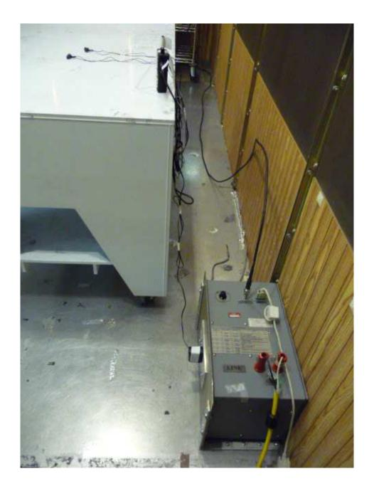
AC Mains Line-Conducted Disturbance Setup Photograph
