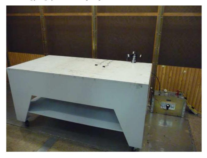
AC Mains Line-Conducted Disturbance Setup Photograph
