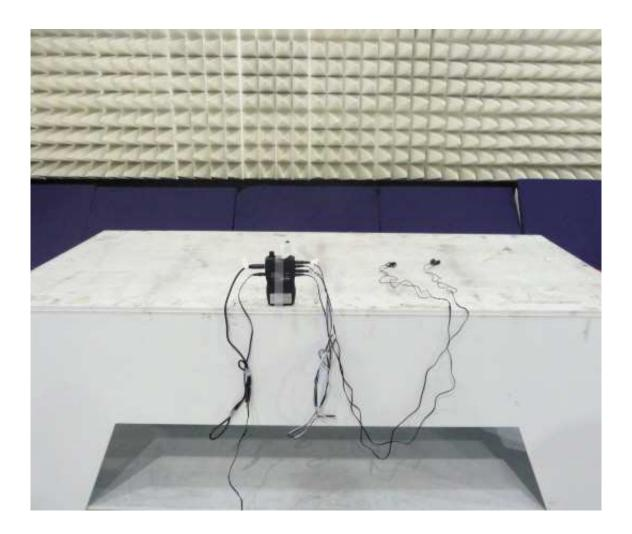
Electromagnetic Radiated Disturbance Setup Photograph
