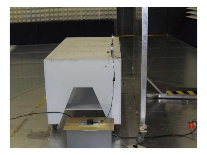
Electromagnetic Radiated Disturbance Setup Photograph
