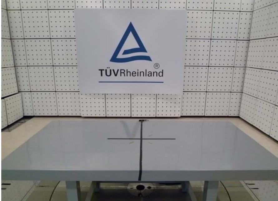
Photograph 2: Set-up for Spurious Emissions (Back View)
