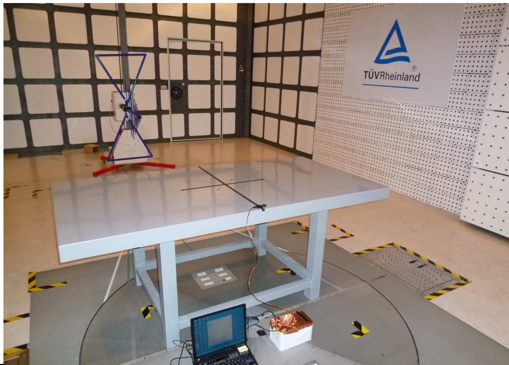
Photograph 2: Set-up for Spurious Emissions (Back View)
