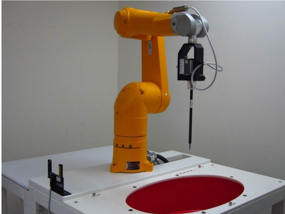
Fig.1 Photograph of the SAR measurement system
