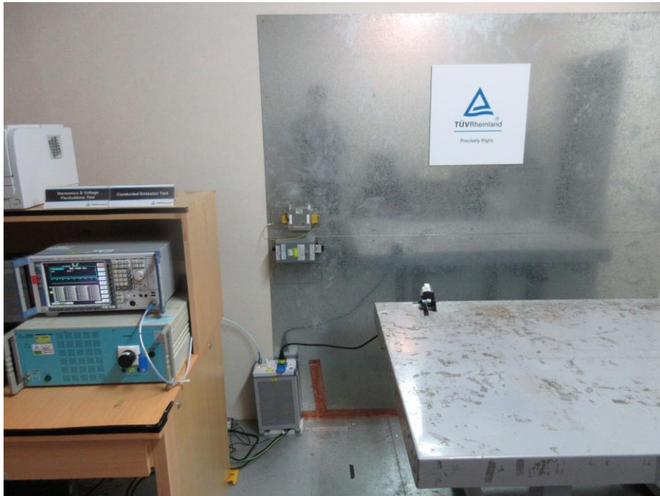
Photograph 7: Set-up for Mains Conducted testing (Front View)
