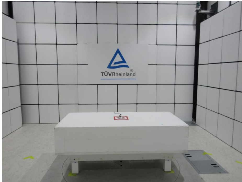
Photograph 1: Set-up for Spurious Emissions (Front View 1)
