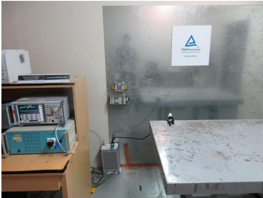
Photograph 7: Set-up for Mains Conducted testing (Front View)
