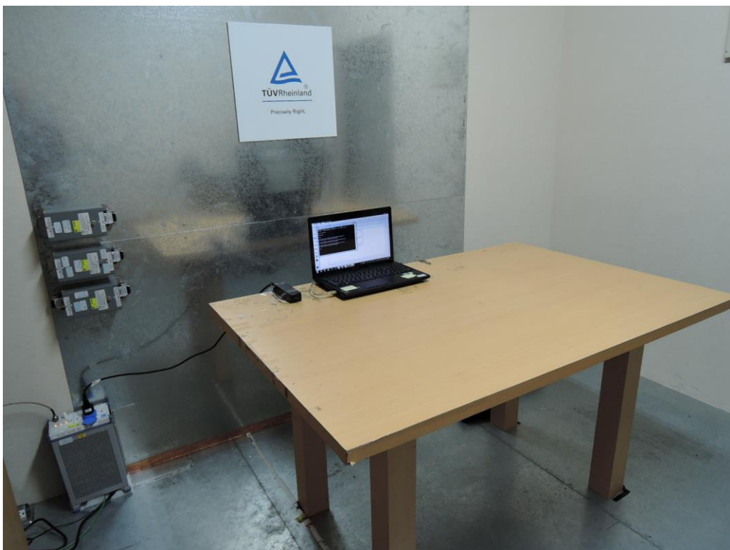
Photograph 6: Set-up for for Mains Conducted testing Front
