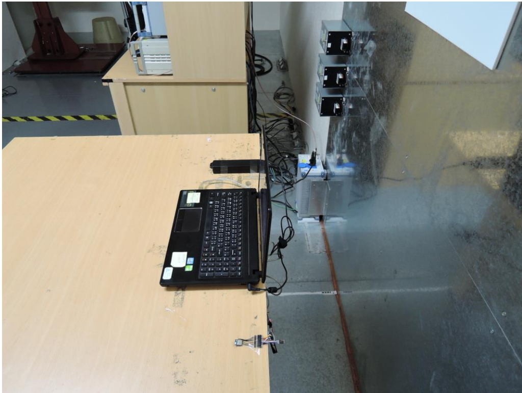
Photograph 5: Set-up for for Mains Conducted testing Back
