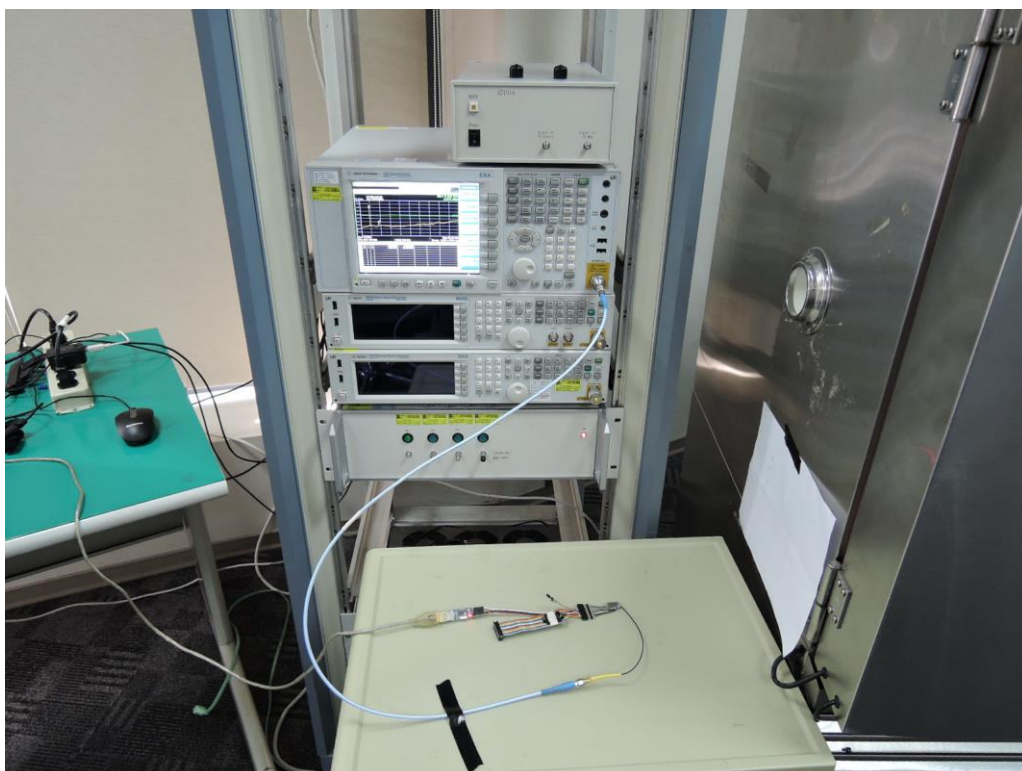
Photograph 4: Set-up for Conducted testing
