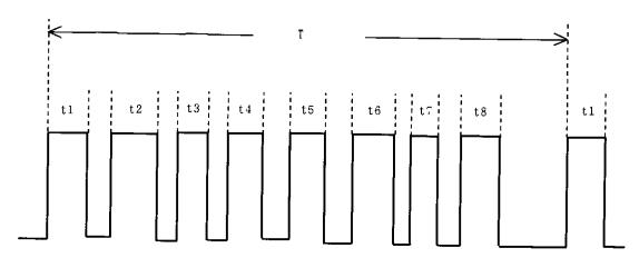
Duty cycle =  $\frac{\text{The value of the sum of the pulse widths in one period } \sum_{n=1}^{8} t_n}{\text{The length of period (T)}}$
