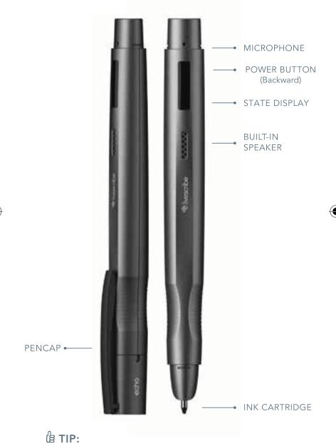
If your smartpen doesn't power on, you may need to charge it. To charge, make sure your computer is on, and connect your smartpen to your computer with the included micro USB cable. A full charge may take up to 2.5 hours.
