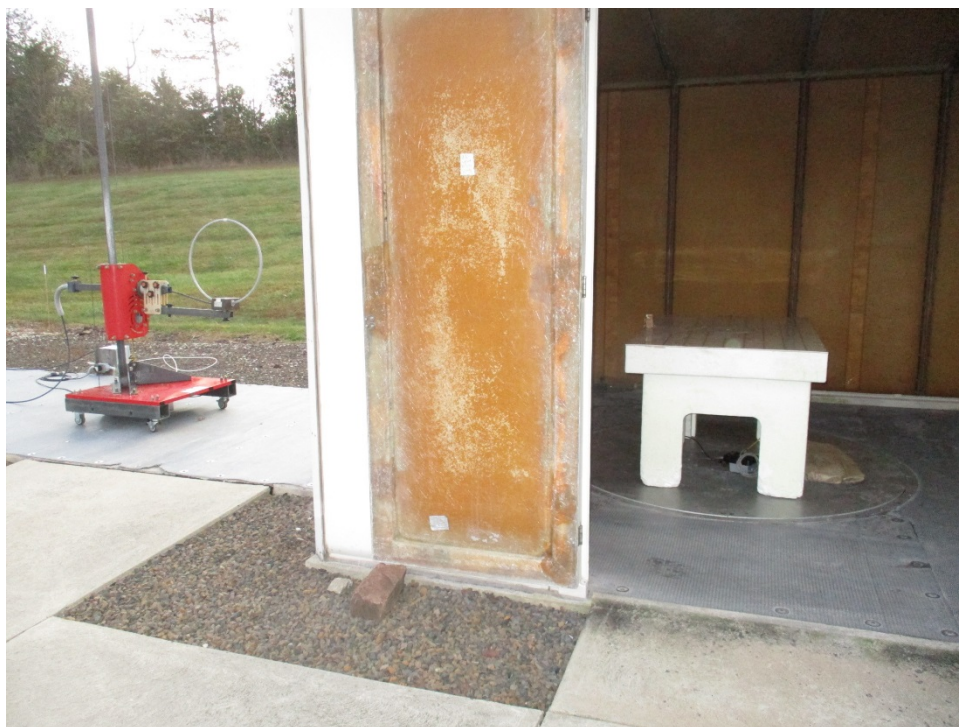
Test Setup, 9 kHz to 30 MHz, Perpendicular
