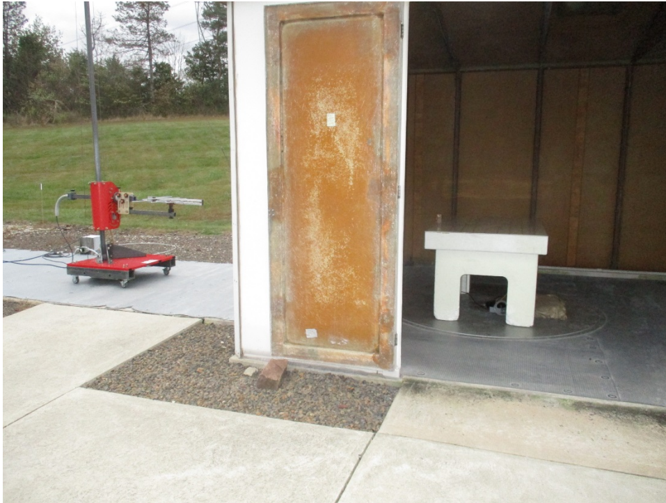
Horizontal Antenna Polarization, 200 MHz to 1 GHz
