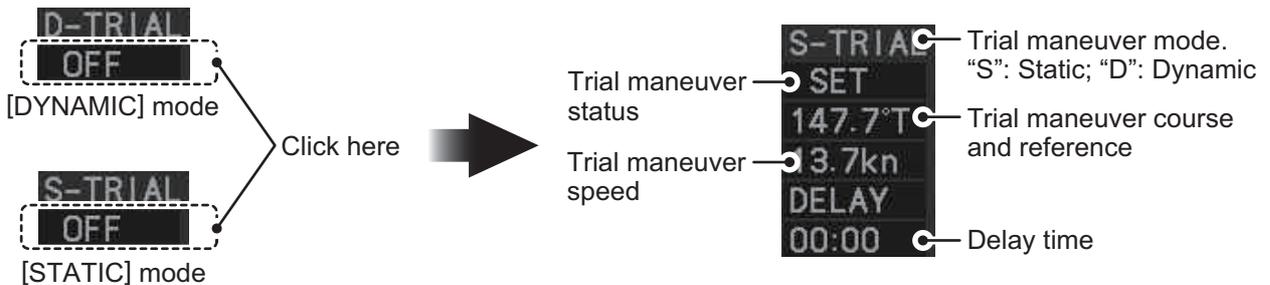
**Note:** The initial indications for course and speed are derived from own ship's current course and speed at the time when the trial maneuver set up starts.
