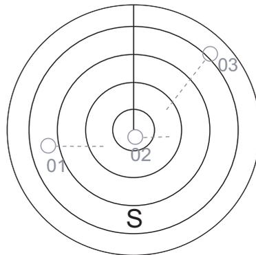
Place the cursor on a target, then press the **ACQ** key to display the target data.
