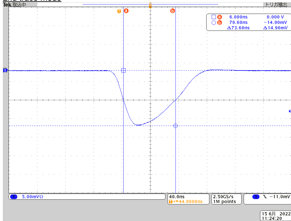
Fig. 6.13 S1 pulse envelope
