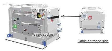
5. Apply the supplied adhesive to the threads of the cable glands, and then fasten it tightly with the hook spanner.
