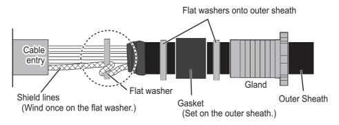
4. Pass the antenna and power cables through each cable glands and attach the appropriate connectors to the appropriate cables. For how to connect the cables to WAGO connector, see "WAGO connector" on page 2-5. For pin arrangement, see the interconnection diagram at the back of this manual.
