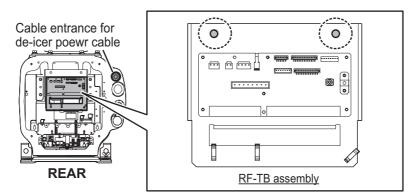
2) Wrap the supplied spiral tube around the de-icer power cable, starting from the crimp-on lugs. Set a locking wire saddle (supplied) at location (5) shown
