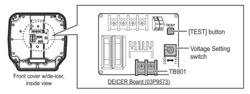
1) Unfasten two bolts to remove the RF-TB assembly, then pass the de-icer power cable through the cable entrance.
