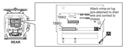
10. **For DE-ICER INSTALLATION**, connect the de-icer power cable the de-icer board 03P9573 attached on the front cover. If the de-icer is not provided, go to step 12.
