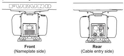
1. Loosen 12 bolts from both covers to remove the covers.
