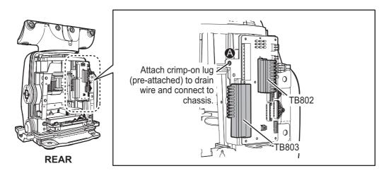
7. **For DE-ICER INSTALLATION**, connect the de-icer power cable the de-icer board 03P9573 attached on the front cover. If the de-icer is not provided, go to step 8.
