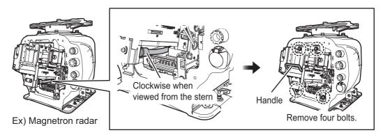
4. Remove the RF unit with the handle.
