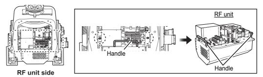
**Note:** The magnetron in the transceiver module will demagnetize if it contacts ferrous material. When dismounting the transceiver module, lay it on its side or on top of non-ferrous material as shown in the figure to the right.
