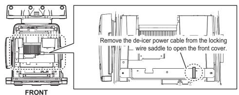
**Note 2:** For the de-icer, take care not to hit the heater elements on the chassis or radiator. If the heater hits something, unfasten the fixing screws for the heater to adjust the position of the heater. Then fix the heater again.
