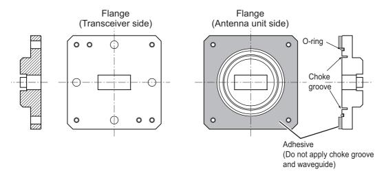
4) Connect the waveguide flange and then fix with the bolt.
