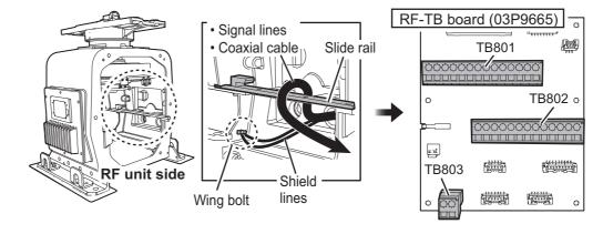
3) Remove the TNC junction box from the RF unit and then connect the coaxial cable of the antenna cable to the BNC case.
