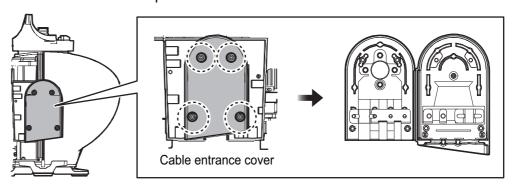
**Note:** The orientation of the cable entrance can be changed. See "How to change the orientation" on page 2-11.
