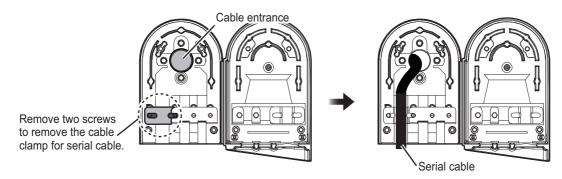
If applicable, unfasten the two screws fixing the cable clamp for the de-icer power cable, then pass the cables through the cable entrance.
