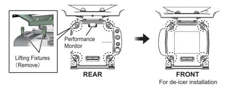
**Note 1:** The cable for the performance monitor is connected between the rear cover and the RF-TB Board in the Antenna Unit. Open the cover slowly to prevent damage to the cable and connector.
