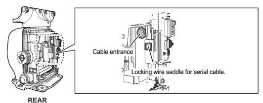
6. Attach the appropriate WAGO connectors (pre-attached) to the serial cable, and then connect the serial cable to the RF-TB Board as shown in the following figure. For how to connect the WAGO connector, see "WAGO connector" on page 2-5. For pin arrangement, see the interconnection diagram at the back of this manual.
