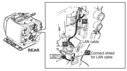
**Note:** For the antenna cable RW-9600/6895/4873, connect the crimp-on lug (that binds unused wires) together with the shield of the power line.
