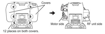
**Note 1:** If the performance monitor is installed, the cable for the performance monitor is connected between the cover for the RF unit side and the RF-TB Board in the Antenna Unit. Open the cover slowly to prevent damage to the cable and connector.
