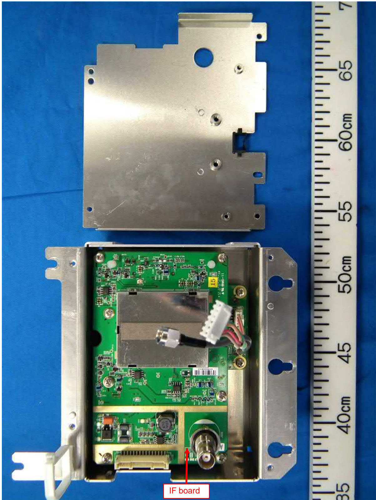
1.12 IF board 03P9666 and IF-TB board 03P9711 module (with the metallic cover removed, showing IF board 03P9666)
