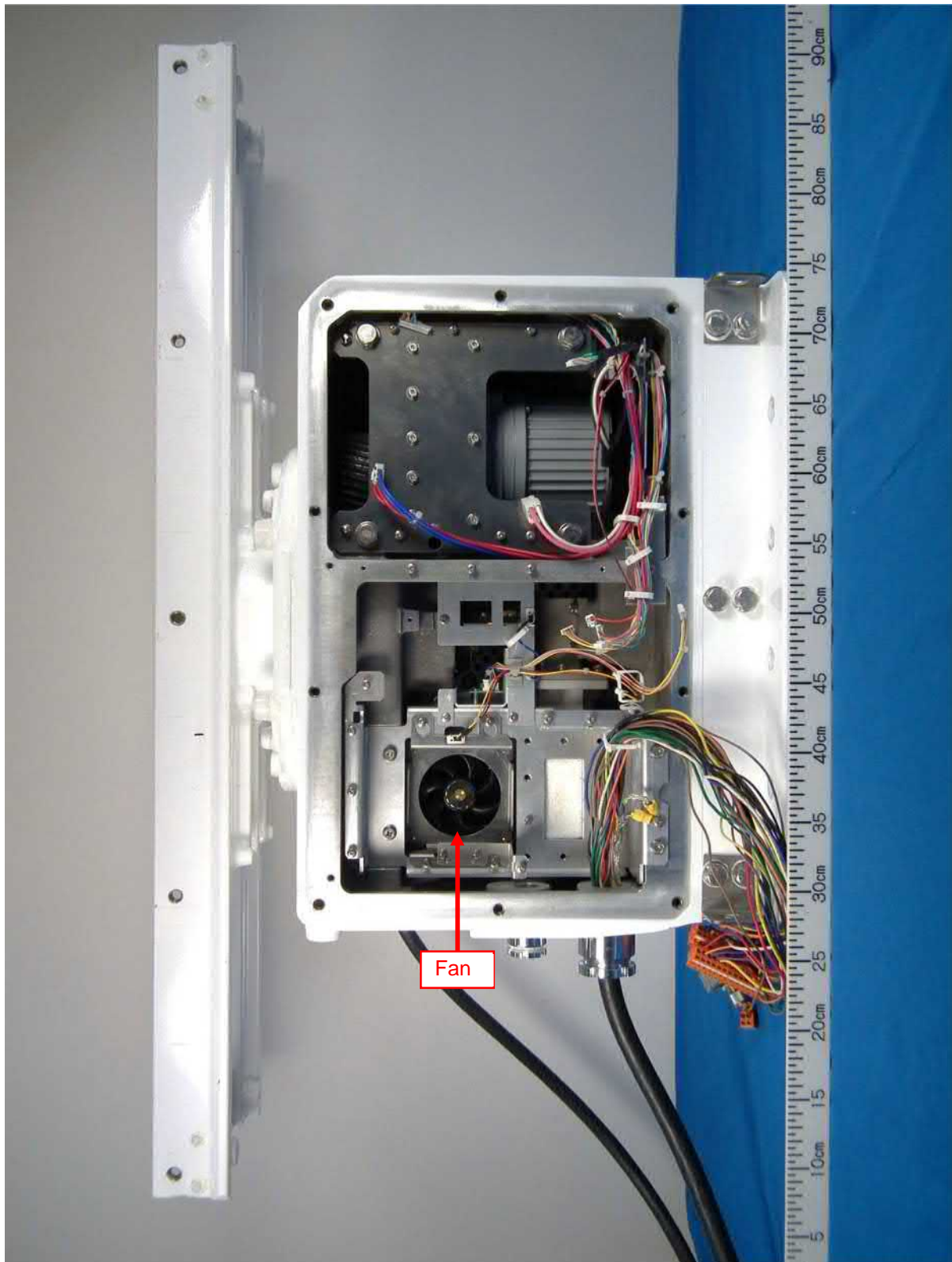
1.14 Right side view (with IF board 03P9666 and IF-TB board 03P9711 module, and the metallic base part removed, showing the fan)
