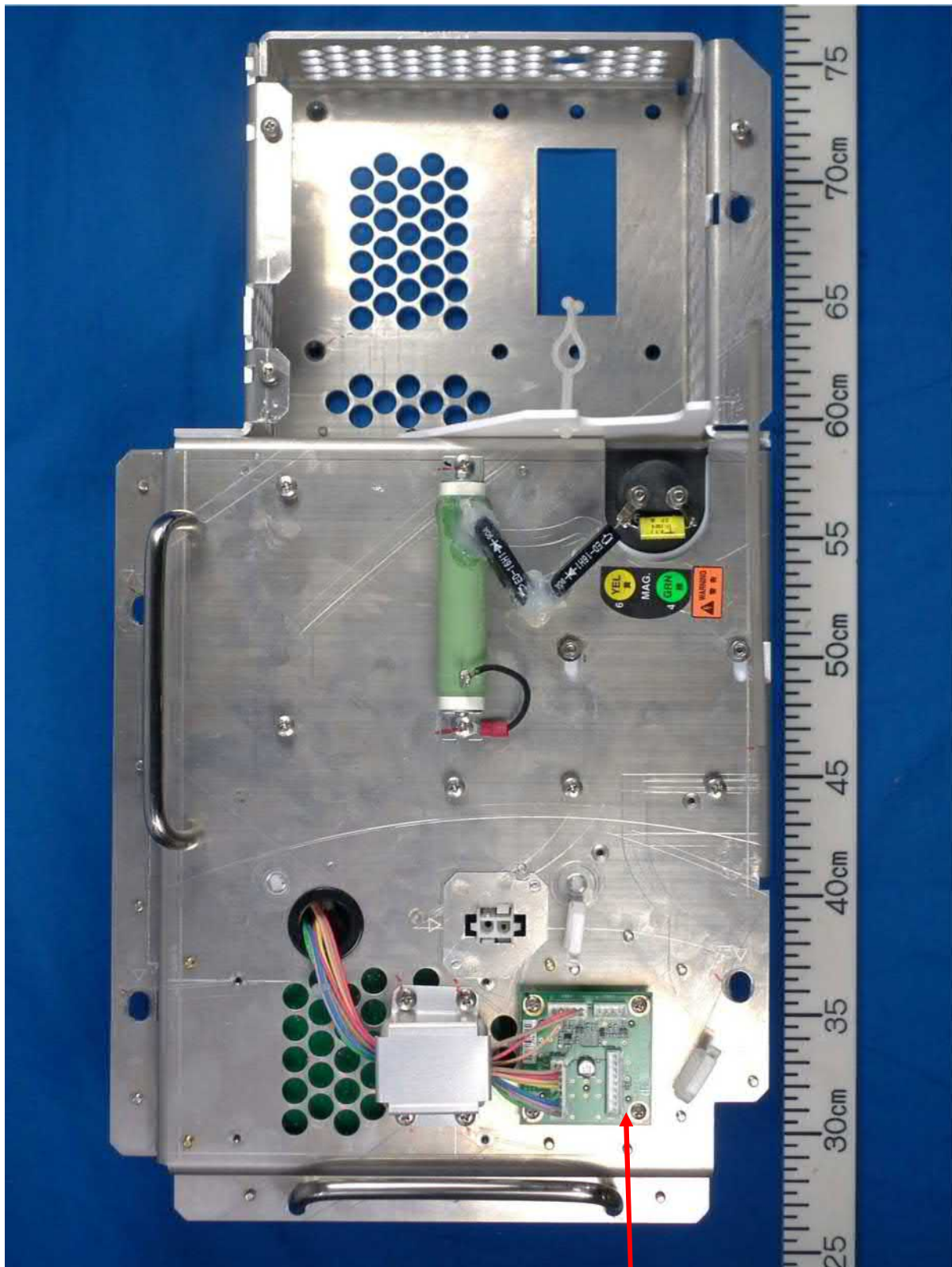
1.19 Transceiver RTR-129, Front side (showing BUF board 03P9446)
