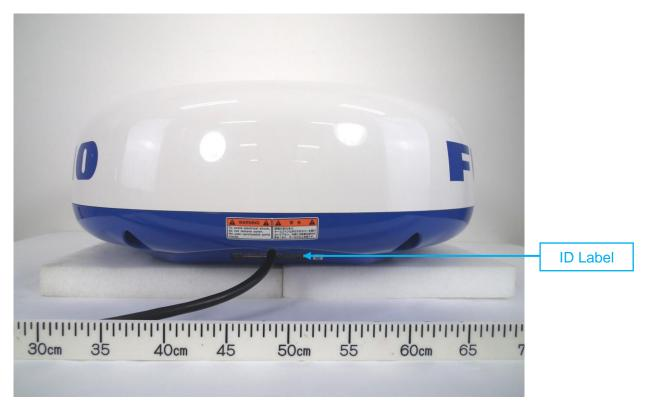
ID Label is affixed on the scanner case of RADAR SENSOR.
